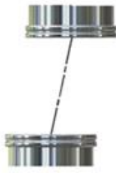
Off Set equipment IG = CL - 20mm (Minimum)
