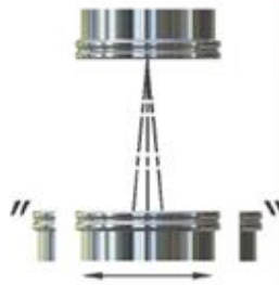
Oscillating equipment IG = CL - 40mm (Minimum)
