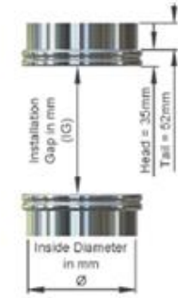
In-line static equipment IG = CL - 10mm (Minimum)
