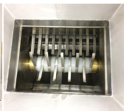
Removable breaking finger, Option for cutting feature
