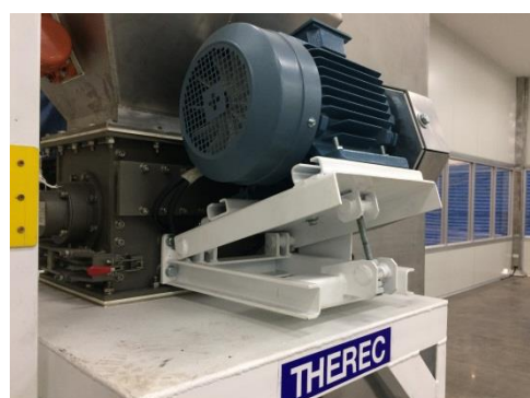
Adjustable motor base for belt tensioning
