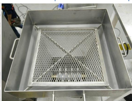
Safety screen for low loading hopper
