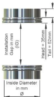
In-line static equipment IG = CL - 10mm (Minimum)
