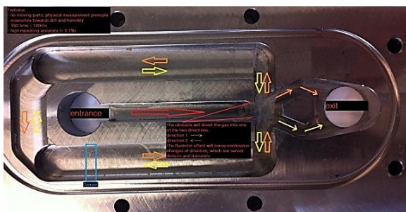
Oscillating Principle of Measurement
